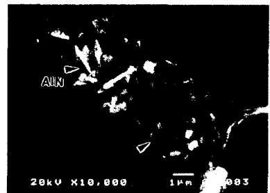
Fig. 6 SEM Micrograph showing reaction products, AIN, after dissolving away Al alloy matrix (9)
