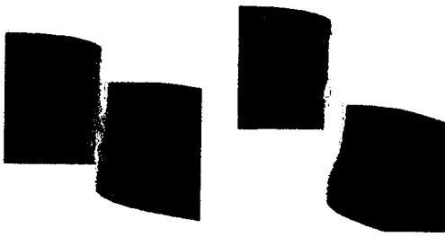
(a) Before fracture (b) After fracture Fig. 10 Plastic strain 2.0 (clearance 0.03mm)
