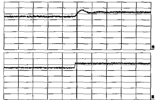
Fig. 12 Output voltage waveform of the parallel PWM converter varying the reference voltage (X-axis : 0.2 s/div , Y-axis : 65V/div)
