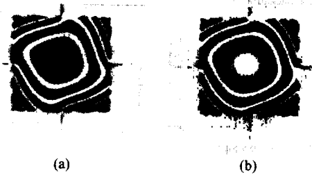
Fig. 14. Fringe patterns observed at the 250 \times 250 \mu\text{m}^2 micromirror under no bias (a) and 5 V DC bias applied at the PZT cantilever unimorphs (b).
