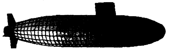
Fig. 5. Exterior flexural energy density ( f=2kHz, \eta=0.01 )
