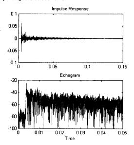
The wide range of available orders allows the identification of varying responses and adaptability to the measurement. An additional possibility is the calculation of two impulse responses from the same excitation, which allows the application of several methods of determining binaural transfer functions based on the use of an artificial head. An example of a classical method and its wide-band echogram (time zoom) is presented here.
