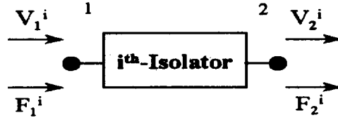
Fig. 3 Input-output relation in uni-directional single isolator.
