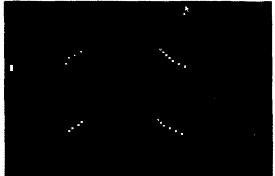
그림 6. 2-dimensional phase cyclic diagram of partial discharge shown in Figure 5. Resembles a typical partial discharge generated from floating electrodes.
