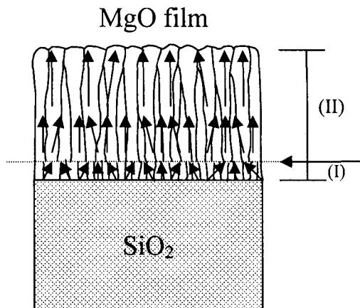
Figure 1. Schematic representation of the microstructural development of MgO films deposited on SiO<sub>2</sub>. The arrows in the MgO columns represent the <111> orientations.
