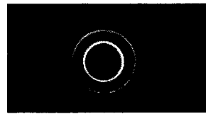
(a) CIMDO V_d=17.91 [kV], I_d=8.64 [mA]
