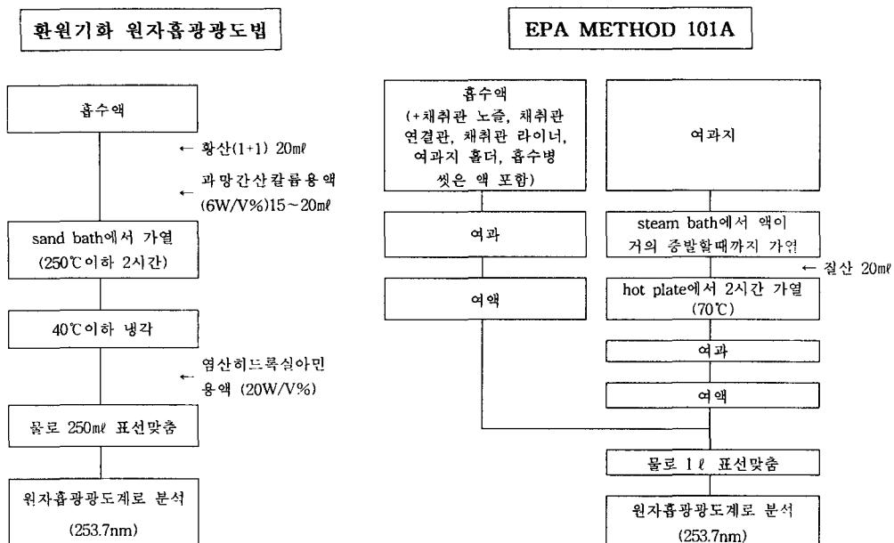
Fig. 1. Flowchart of cold vapor atomic absorption spectrophotometry analysis and EPA Method 101A for measurement of mercury in the flue gas
