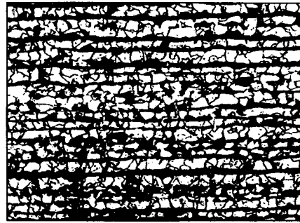
Fig. 5 Microstructure of grade 'AH' steel plate with cold formed.
