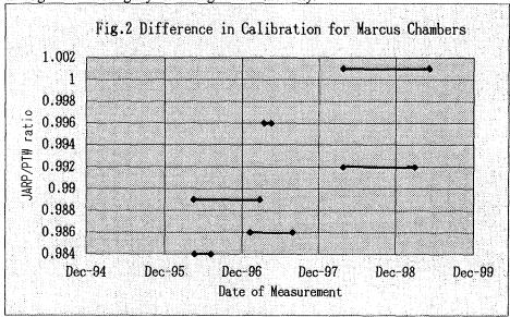
**Discussions:** It seems that the JARP/PTW ratio is becoming unity. It is most likely that the calibration factors by PTW have been modofied gradually, as we have not changed the calibration factors of the standard JARP chambers, nor the protocol to derive absorbed dose from the exposure measurements. We need more data to confirm these observation and also we need discussions with PTW on this issue.
