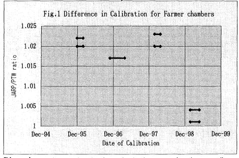
**Discussions:** It became clear that there existed rather systematic and constant discrepancies in exposure calibration factors between PTW and Japanese centers. In 1999, however, JARP/PTW ratio became unity. It is most likely that the calibration factors by PTW have been modofied, as we have not changed the calibration factors of the standard JARP chambers. We need more data to confirm these observation and also we need discussions with PTW on this issue.
