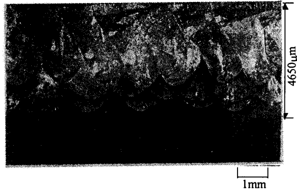
Fig. 1 Macrography of GBM Cross-Section by electron beam
