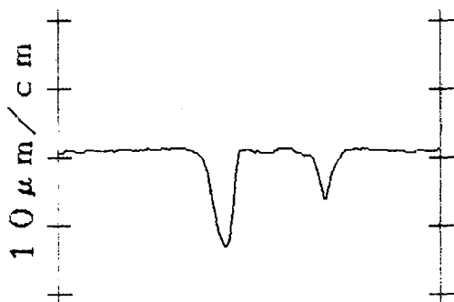
Fig. 8 (b) Profile curve of a worn surface (Zircaloy-4, 40\mu\text{m} , 100N, 3 \times 10^5 cycles)
