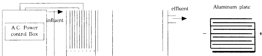
Fig. 1. Schematic diagram of electrocoagulation apparatus
