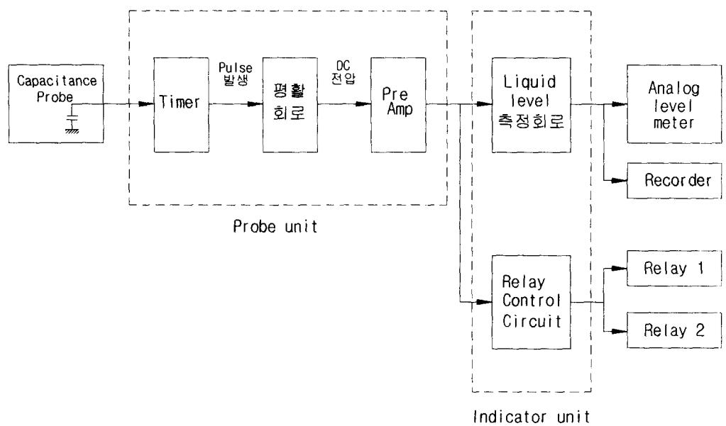
Fig. 2. The block diagram of level meter circuit.
