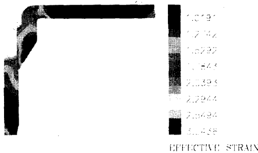
Fig. 10 Distribution of effective strain for 2 stage forging process
