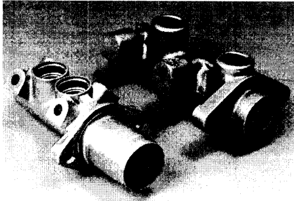
Fig. 1. Thixoformed master cylinders (fabricated by thixoforming (left) and permanent mold casting (right)) show better near net shape.
