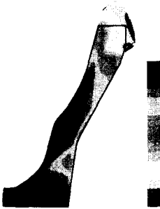
Fig.11 Distribution of fracture values for final forging I (Bold line is configuration of final product)
