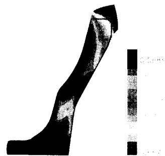
Fig.10 Distribution of fracture values for final forging
