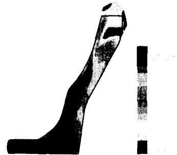
Fig.13 Distribution of fracture values for final forging III (Bold line is configuration of final product)
