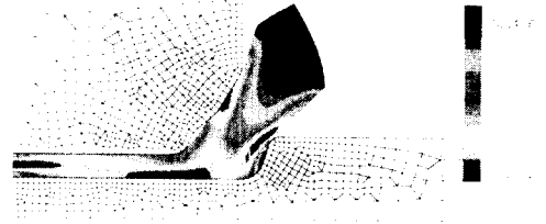
Fig.7 Distribution of effective strain for preforming II
