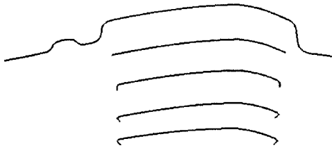
Fig.6 Deformed profile of section y=-301.48
