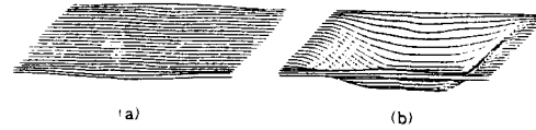
Fig. 12 The second stamping 3D simulation of modified blank for the anisotropic material (a) initial workpiece (b) stroke = 100%
