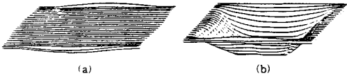
Fig. 8 The second stamping 3D simulation of modified blank for the isotropic material (a) initial workpiece (b) stroke = 100%
