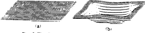
Fig. 3 The first stamping 3D simulation for the isotropic material (a) initial workpiece (b) stroke = 100%
