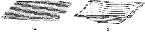
Fig. 5 The first stamping 3D simulation of modified blank for the isotropic material (a) initial workpiece (b) stroke = 100%
