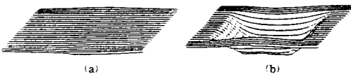
Fig. 9 The first stamping 3D simulation of modified blank for the anisotropic material (a) initial workpiece (b) stroke = 100%
