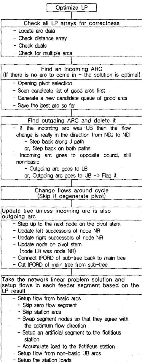
Develops the sequence of segments as if one was walking away from the substations and down each feeder
