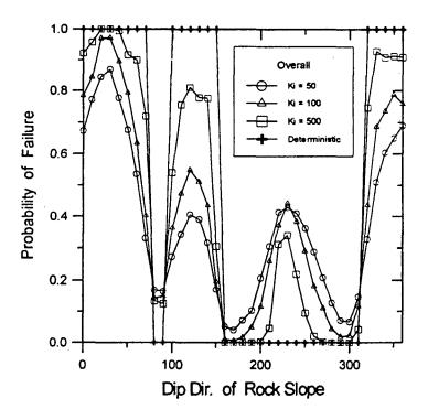
Figure 8:  $P_f$  versus  $\alpha_f$  with the variation of K
