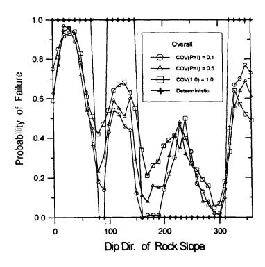
Figure 9:  $P_f$  versus  $\alpha_f$  with the variation of coefficient of variation of  $\phi$
