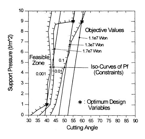
Figure 10: Sensitivity of Optimum Solution to the Change of the Prescribed Failure Probability (when  $\beta_f$ =20°)
