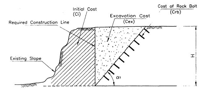
Figure 4: Definition of initial cost, excavation cost, and cost of rock bolt
