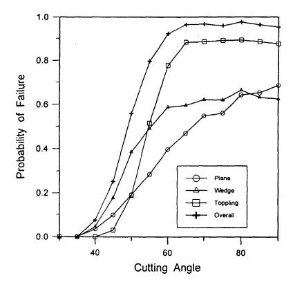
Figure 6:  $P_f$  versus  $\alpha_f$  ( $\beta_f$  =20° and q = 0 t/m²)
