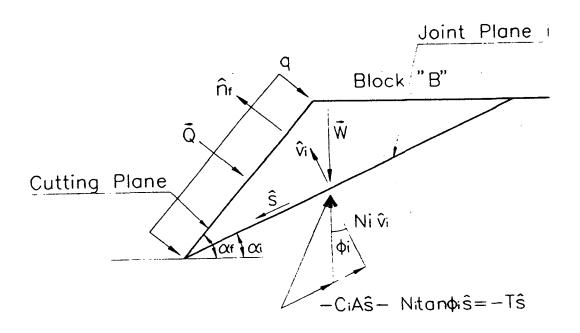
$\hat{n}_i$ : unit vector of cutting plane  $\alpha_i$ : dip angle of cutting plane  $\alpha_i$ : dip angle of joint plane i  $C_i$ : cohesion of joint plane i  $\phi_i$ : friction angle of joint plane i
