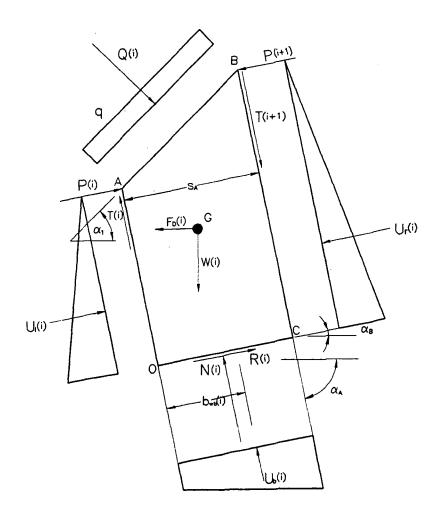
Figure 3: Forces applied to slice (i)
