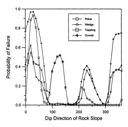
Figure 5:  $P_f$  versus  $\beta_f$  ( $\alpha_f$  =70° and q = 0 t/m²)
