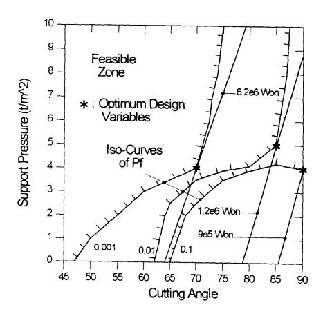
Figure 11: Sensitivity of Optimum Solution to the Change of the Prescribed Failure Probability (when  $\beta_f$  =210°)
