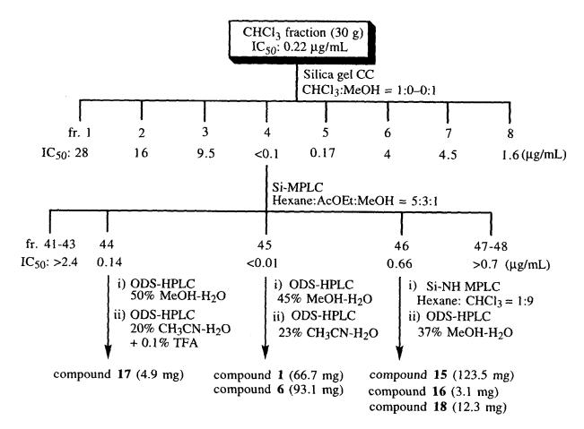
Procedures for Separation of Compounds from CHCl<sub>3</sub> Fraction
