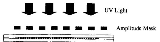
Fig. 1. Schematic diagram of fabrication of sampled fiber grating.
