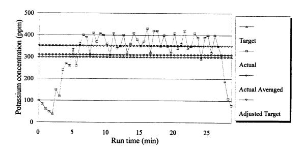
Fig 2 An example of how the fertigator was designed to deliver nutrients and adjust the target concentration to account for run time. The change of actual potassium nitrate concentration from the fertigator during a run time of the fertigator. The water requirement was 300 liters and each 20 liters was programmed for the initial and final clear volumes.
