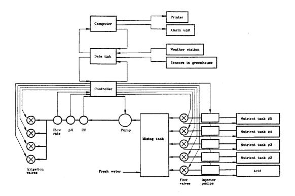
Fig 1. Block diagram of the computerized fertigation system tested in the experiment.
