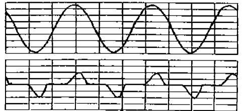
Fig. 10 Output voltage (70V/div, 5ms/div) and load current (12A/div) in back-up power mode.
