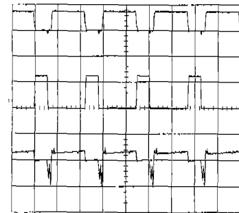
(b) Voltage/current waveforms of the switch S_B in case of large duty cycle D_{TB} :
