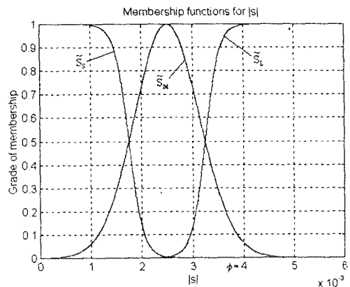
그림 2 퍼지집합 \tilde{S}_S, \tilde{S}_M, \tilde{S}_L Fig. 2 Fuzzy sets \tilde{S}_S, \tilde{S}_M, \tilde{S}_L
