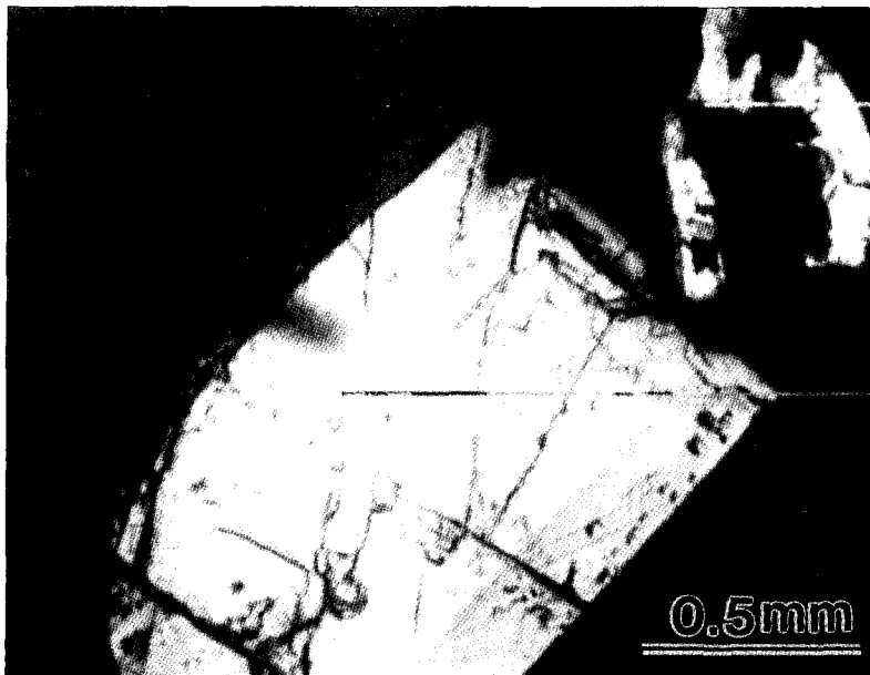
Fig. 2. Polarizing Micrograph of ZnS(Sphalerite) after ion milling.
