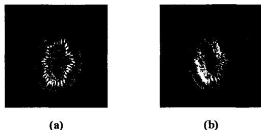
Fig. 3. A kiwi image and its corresponding sinogram obtained by experiment.
