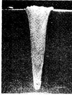
Photo.3 Cross section of weld (A5083-O).
