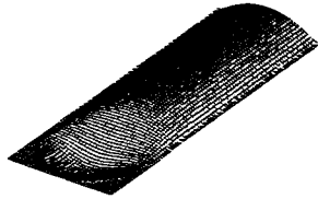
Fig. 4 Calculated weld bead shape
