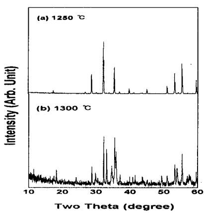
Fig. 1 X-ray diffraction patterns (Cu-K $\alpha$ ) of sintered CuB(1.0 wt%)-YIG
