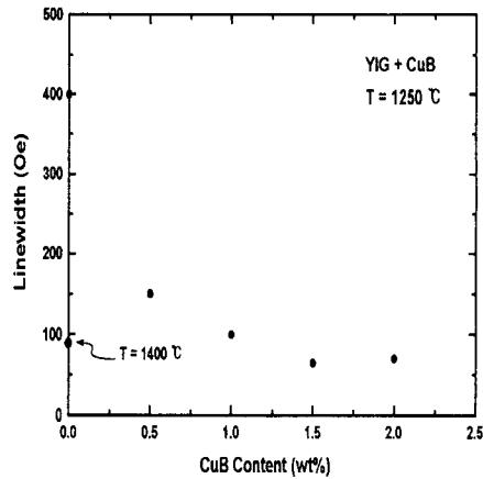
Fig. 2 Variation ferromagnetic resonance line width  $\Delta H$  of YIG specimen sintered at 1250 °C, with CuB content.
