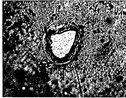
Fig. 2. Optical microscopic photograph at the ambient region around the artificial void filled with humidity before tree initiation.
