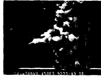
Fig.7 Expelled copper dross around hole
