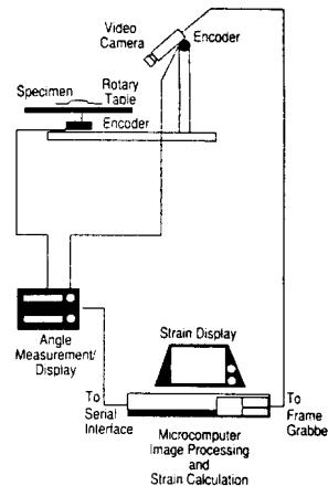
Fig.1 A Schematic diagram showing the major components used in the automated visionbased strain measurement method.
