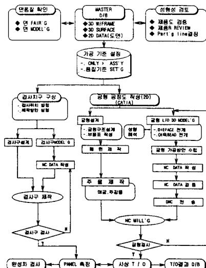
Fig.3 Flow chart of CAM system in automobile dies.
