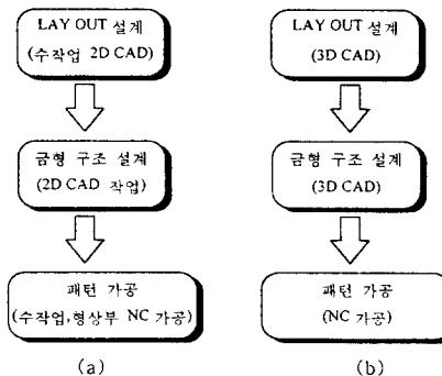
Fig.2 Flow charts of CAD system in automobile dies.
