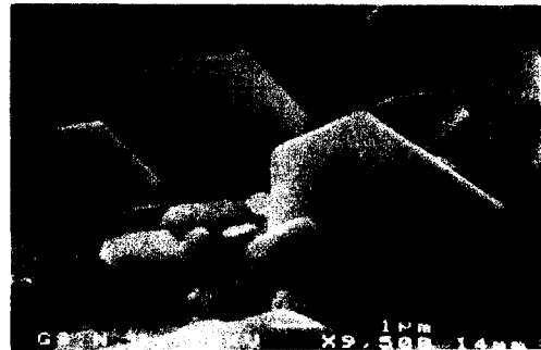
Fig. 5. SEM micrograph showing the shape of WS 2 platelet. The synthesized WS 2 platelet were formed as well-defined hexagonal plates.
