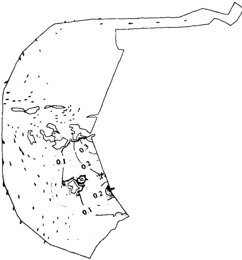
Fig. 3 Velocity and concentration : CASE 1, ebb, time = 159.0 hr.
