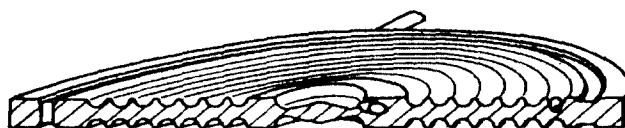
Fig. 2. Spiralplate with half-nine coils for retentate
