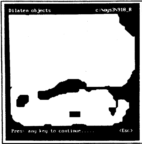
Figure 5. The image resulting after applying the object dilation process to the image in Figure 4.
