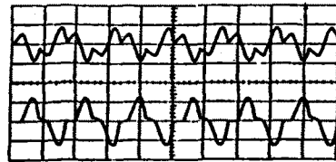
Figure 8: Experimental results of compensation current and load current in APF mode
