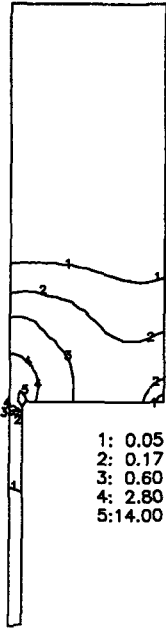
Fig. 5 Distribution of effective strain rate
