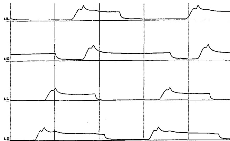
Fig. 2. Current shape of YGN3&4 during insertion of control rod
