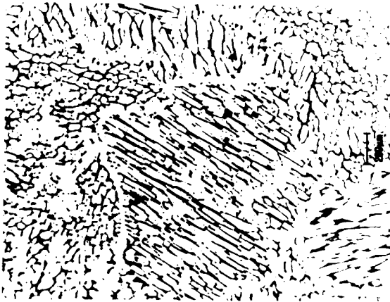
Fig.1 Ferrite morphology of CF8 duplex stainless steel.
