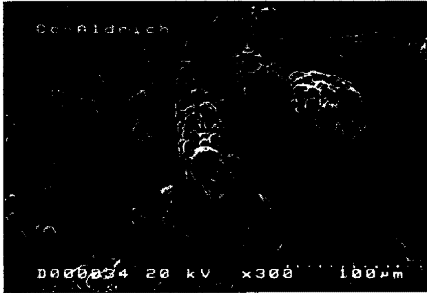
Fig. 2 SEM micrograph of Co skeleton sintered at 900°C, 2hr, H 2 atmosphere
