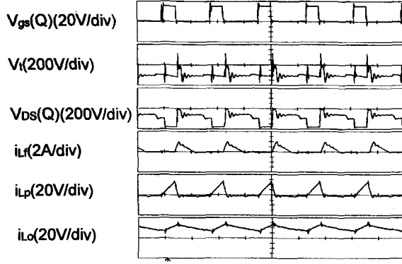
Fig. 8 Experimental waveforms of the proposed converter operating at 60V dc input.
