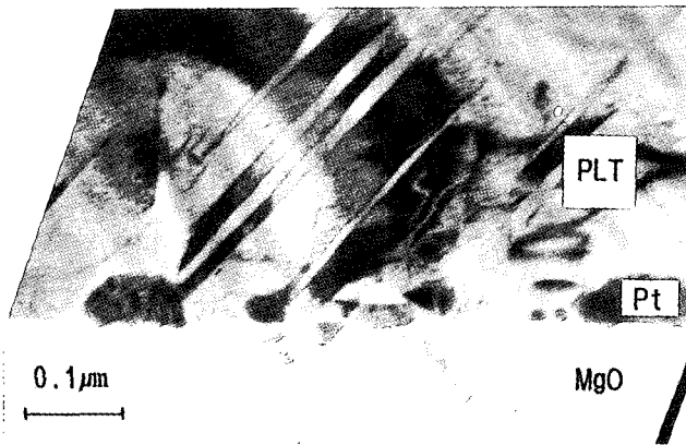
Fig. 1 cross-sectional TEM micrograph of PLT/Pt/MgO
