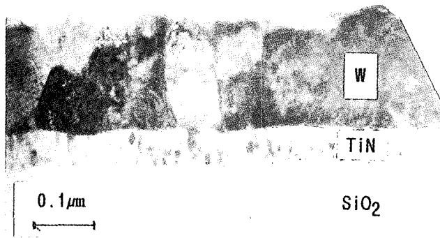
Fig. 3 cross-sectional TEM micrograph of W/TiN/SiO 2 /Si
