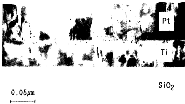
Fig. 2 cross-sectional TEM micrograph of Pt/Ti/SiO 2 /Si
