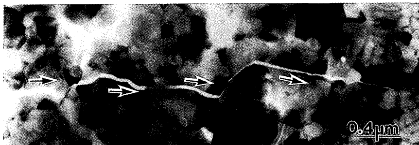
Fig. 3 TEM image showing crack propagation in the \text{Al}_2\text{O}_3\text{-ZrO}_2(8\% \text{Y}_2\text{O}_3) composite.
