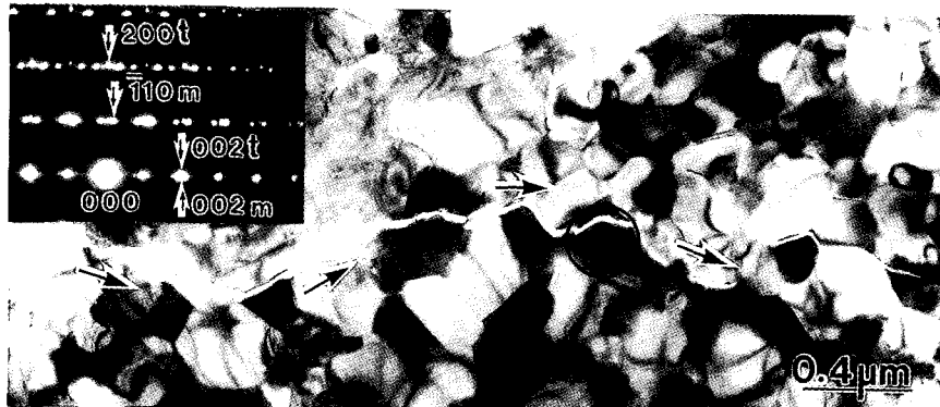
Fig. 2 TEM image showing crack propagation in the \text{Al}_2\text{O}_3\text{-ZrO}_2(3\% \text{Y}_2\text{O}_3) composite. An insetted electron diffraction pattern was taken from the region of a dark circle.
